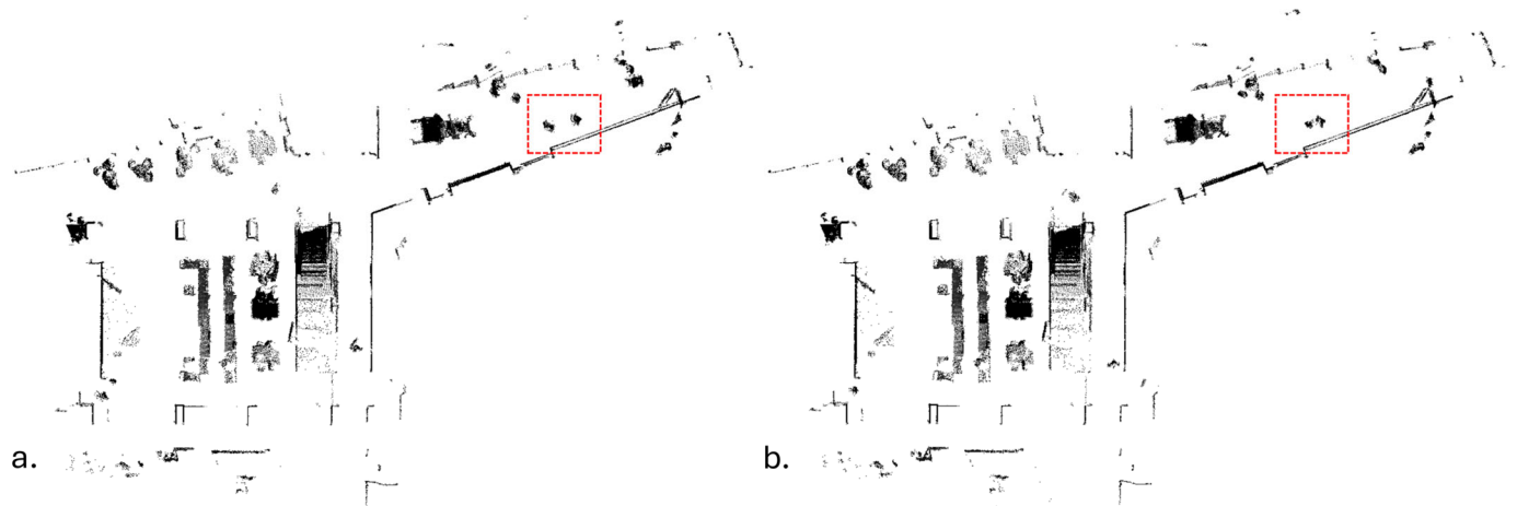
Figure 5. Two orthographic views of maximum intensity-rendered lidar frames overlaid with the collision algorithm. In frame (a), two people are approaching one another (dashed box). In frame (b), they stop and interact—the algorithm successfully detected this collision.
